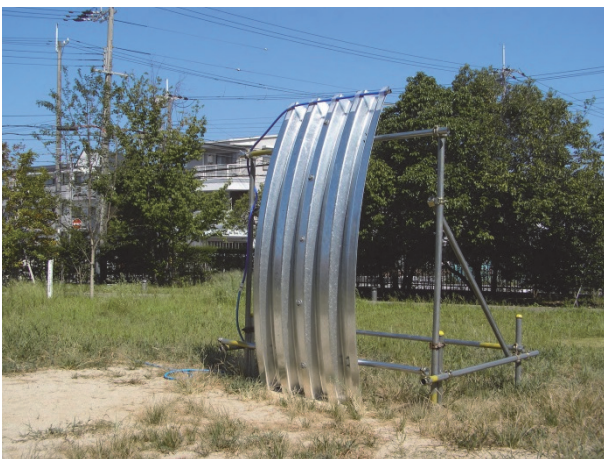
Figure 19. Plank sheet mock-up
